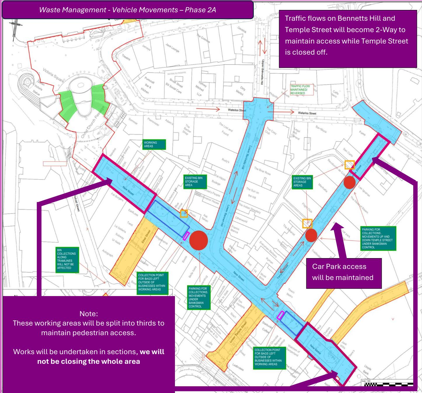
Blue-shaded streets represent **live construction zones** where both delivery and waste-management vehicles will operate under **controlled movement**.
