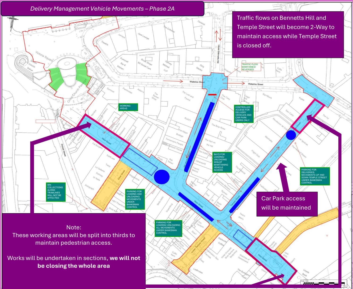
Deep-blue shaded zones (rectangles and circles) represent **loading/unloading bays – all parking will be suspended and loading/unloading only allowed.**
